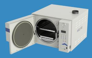
The APOLLON series high-pressure steam sterilizers, manufactured by HANSUNG Co., Ltd. are medical devices that sterilize bacteria, fungi, viruses, and other microorganisms in solid, hollow, porous, and permeable products using saturated steam at high temperatures ranging from 121°C to 134°C and high pressures from 1.1 bar to 2.1 bar, in accordance with the EN 13060 guidelines.
